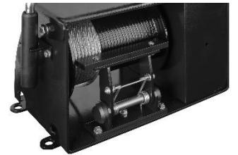
All the nuts of the mounting bolts must be evenly fastened and secured.
