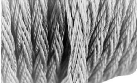
Superflex Plaited Steel Cable is a steel cable of plaited configuration, not laid or twisted like wire rope. The interplaiting of the sets of strands, creates a very tough and set-resistant cable composed of many more wires than is possible with a laid wire rope.
